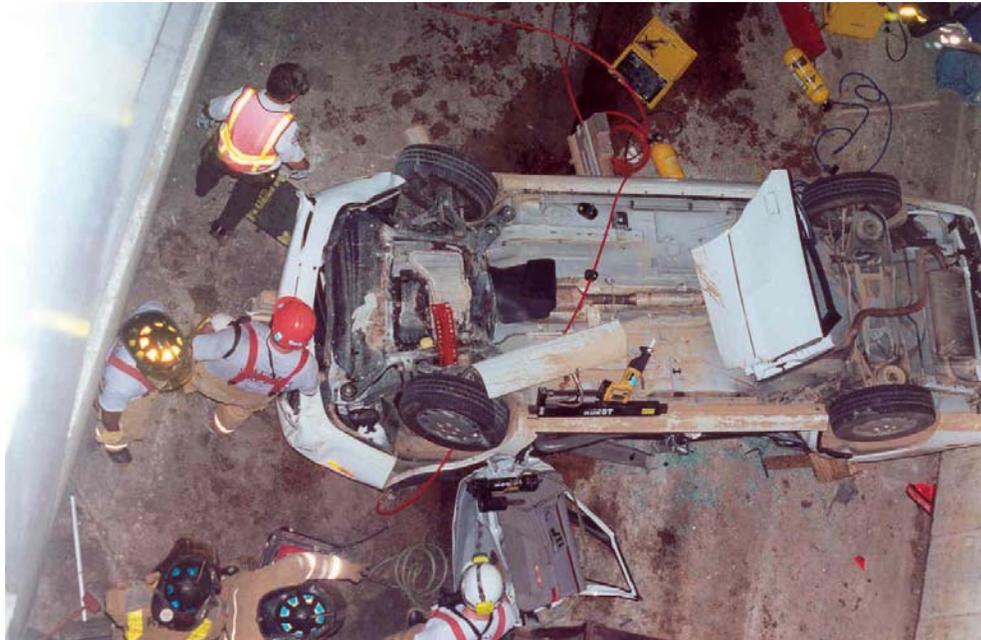
*Fig. 7 This driver floored the accelerator and drove off a parking garage. This type of accident is common. It is known as a Sudden Acceleration Incident (SAI).*
