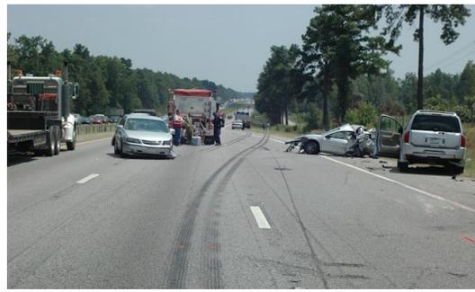
The tractor trailer evasive maneuvering allowed a speed calculation from the geometry and a timing analysis
