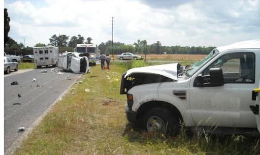
An engine module download gave a detailed description of this truck's speed as it approached collision
