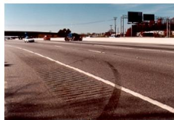
The nature of the tire mark can provide useful information about an accident. A skidmark with bold outside edges is an indication of an overloaded tire. This occurs on the front tires because of the weight shift during hard braking. Skidding rear tires would more likely exhibit a bold center, a characteristic of an underloaded tire.
